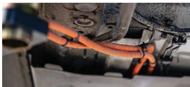
Position of the main circuit breaker under the bonnet and the orange high-voltage cables. Photo: Danish Emergency Management Agency
