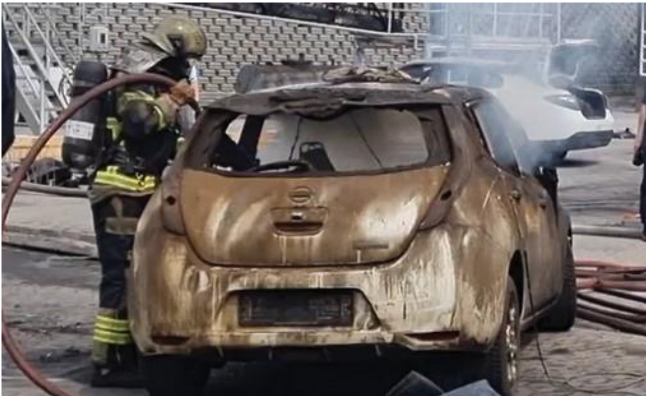
Cooling of battery in the ELBAS project, 2022 Photo: Danish Emergency Management Agency
