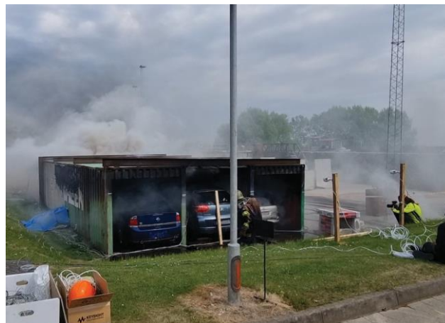
Photo 2: The fire in the battery pack is rapidly increasing and the fire spread to the cabin has started.
