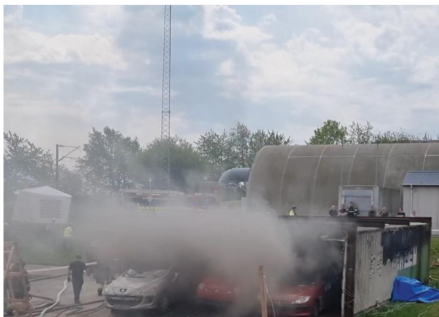
Photo 1: Fire in the battery pack; the smoke is typically white, with slight tinges of brown.
