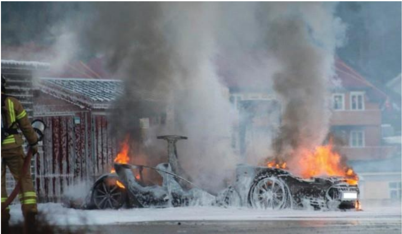
In a fire in a Tesla during charging on 1 January 2016 in Brokelandsheia in Norway, a fire broke out in the high-voltage battery of the electric car. The fire lasted 23 hours and the car was completely burnt out. After the extinguishing efforts were over, 400V high voltage was still present in about ¼ of the battery.
