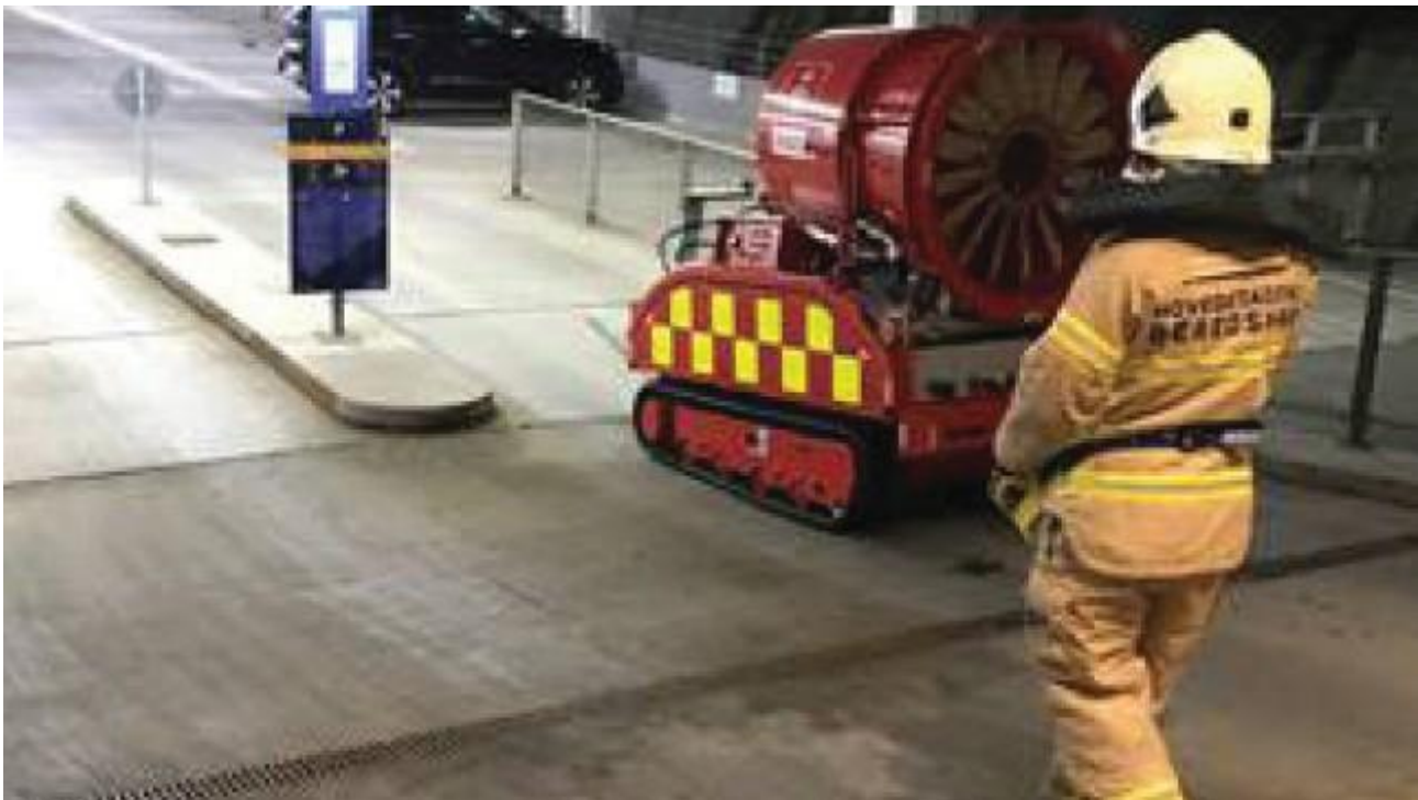
Use of LUF 60, for ventilation and towing of an electric vehicle from underground car parks or parking garages Photo: Hovedstadens Beredskab
