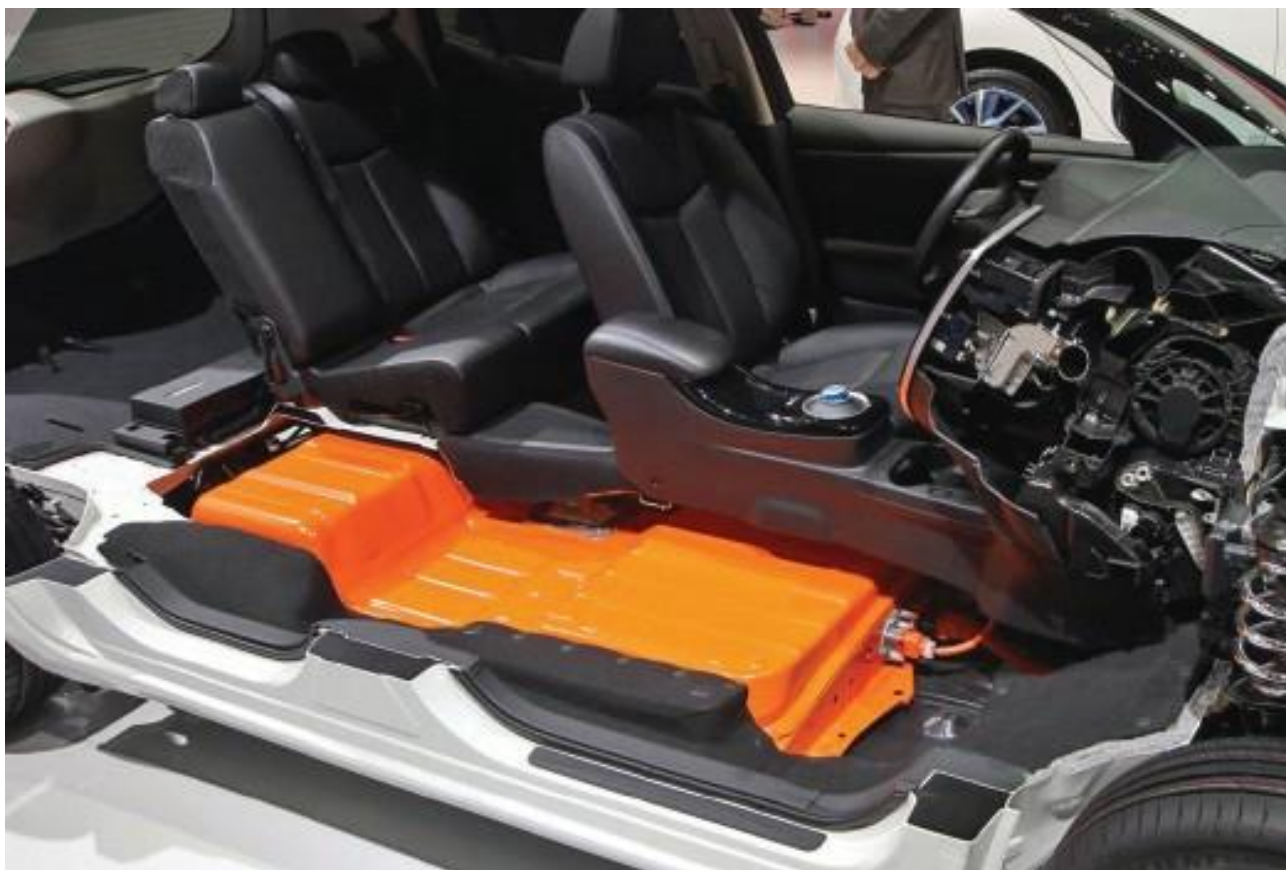
Battery frame integrated under seats in the cab. Photo: Toyota
